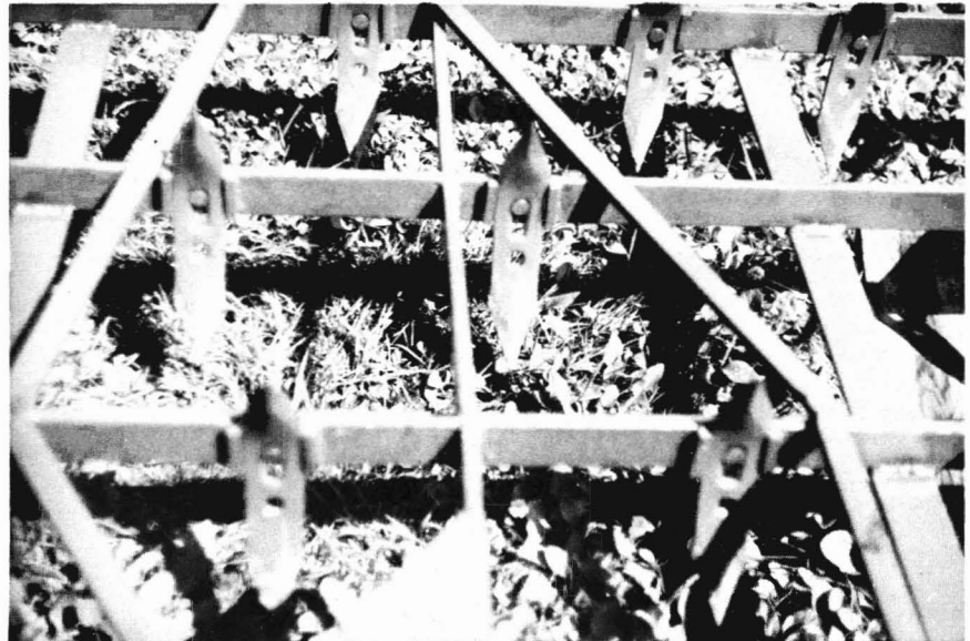
Figure 11.—A cultivator for moving buried shells to the surface of seed beds. The cultivator has four rows of rigid tines which are staggered; the tines are adjustable and reversible. The cultivator would be towed at 3-4 knots, and might have to be fitted with a pressure board to hold it down. A typical oyster dredge boat has the size and power to pull 2-6 cultivators, each about 2.4 m (8 feet) wide.
