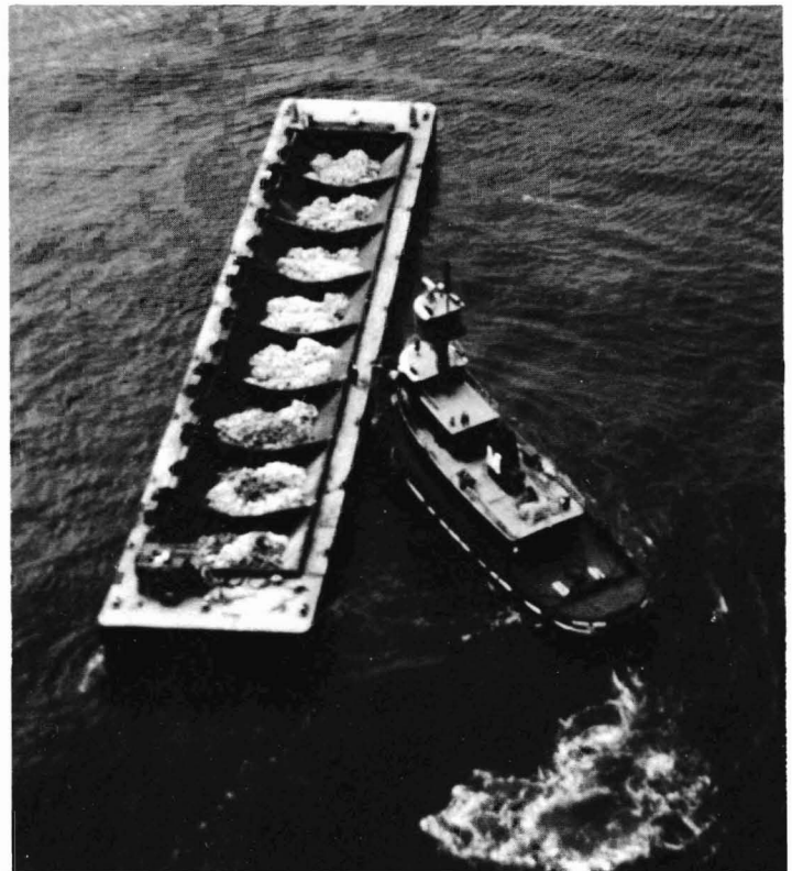
Figure 2.—Barge filled with 15,000 blocks being maneuvered for release at project site.
