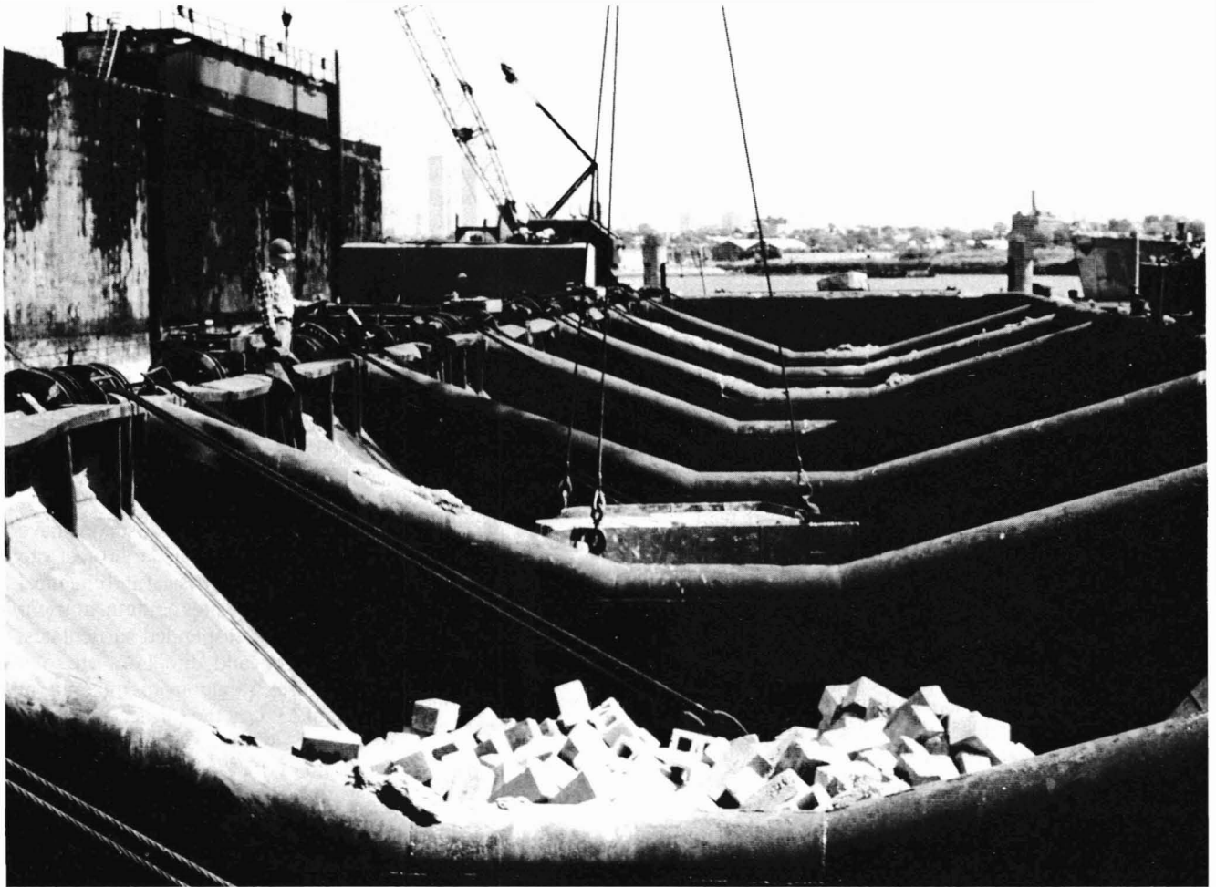
Figure 1.—Loading “pocket” barge with eight compartments fitted with bottom opening doors.
