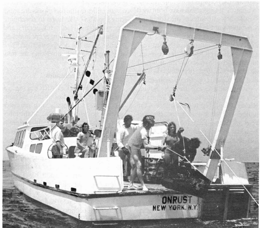
Figure 7.—Shooting a string of fish traps over the stern of SUNY research vessel Onrust .
