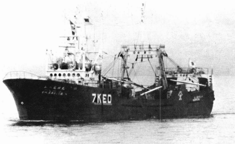
Figure 3.—The Ryujin Maru No. 8 , typical of the class of small Japanese freezer trawlers that fish in the Gulf of Alaska.
