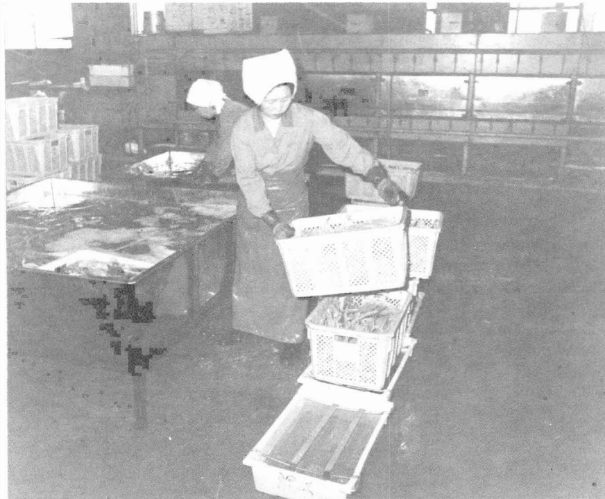
Figure 3.—Squid are removed from cooling bath after skinning (press roaster in background)
