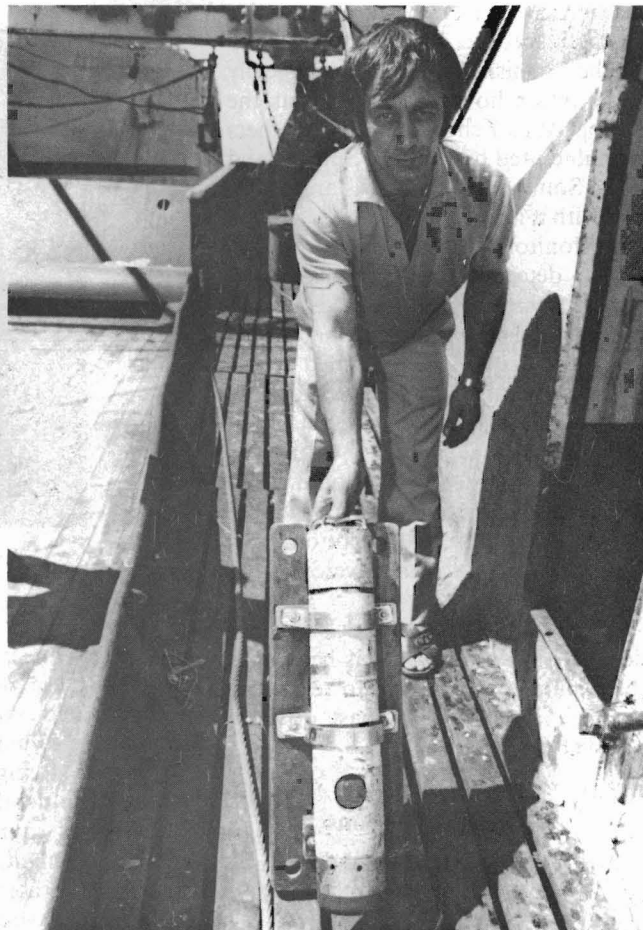
Figure 9.—Battery powered transducer for Koden net monitor.
