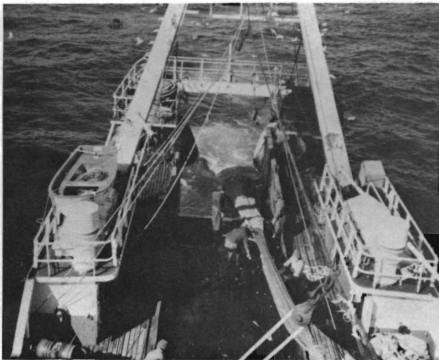
Figure 12.—Taking another bight to haul the cod end on board a Spanish trawler.
