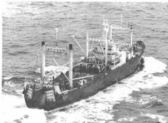
Figure 4.—Japanese stern trawler built in 1964, 84 m in length.
