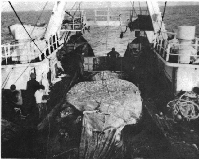
Figure 16.—Five and a half metric ton haulback on a Spanish stern trawler in the Loligo fishery.
