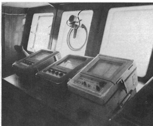
Figure 10.—Two Furuno echo sounders and a Koden net monitor.
