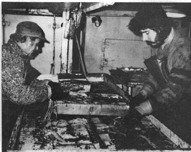
Figure 19.—Packing Loligo in 26-kg trays on Spanish trawler. The two doors in the background are 2 ton flash freezing units.
