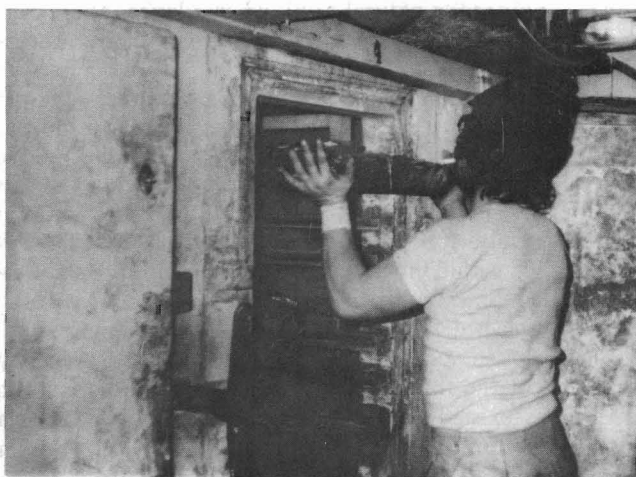
Figure 21.—Italian crewman sliding a 16-kg tray of Loligo into a flash freezing unit.
