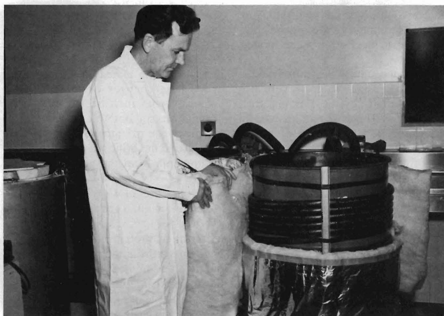
Figure 2.—Brine chiller unit for shrimp-holding experiment. Refrigeration unit is at left. Epoxy-lined holding tanks with plastic cooling coils used to chill the tanks are being covered with insulation.
