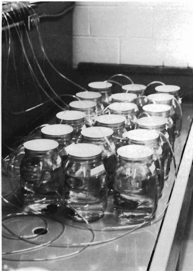
Figure 1.—Exposure system for short-term static tests.
