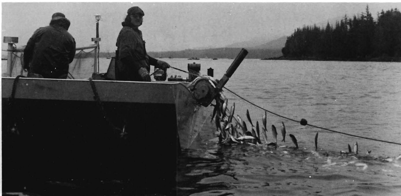
Two fishermen in a Canadian-built skiff haul their set with the aid of a hydraulic net roller.
