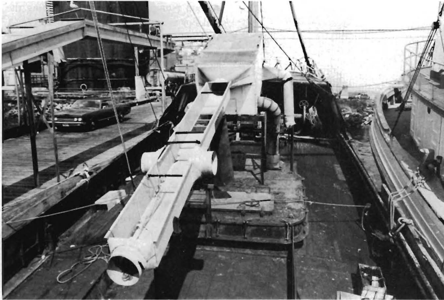
Dewatering box and chute system on the Lady Esther III used in typical New England herring seining operations.
