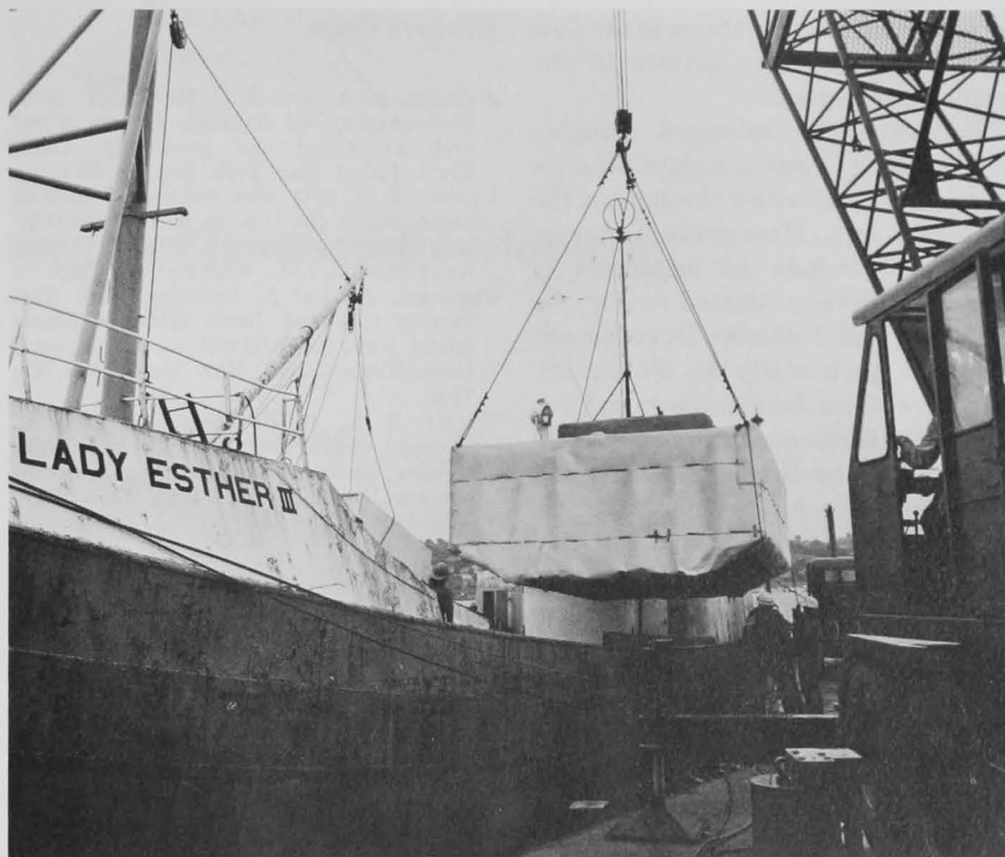
Figure 6.—An insulated container is lowered into a herring carrier vessel. The use of chilled seawater (CSW) has extended the period that herring can be held from less than 12 hours to over 36 hours. This has opened the potential for harvesting herring stocks from a wider geographic range than before.
