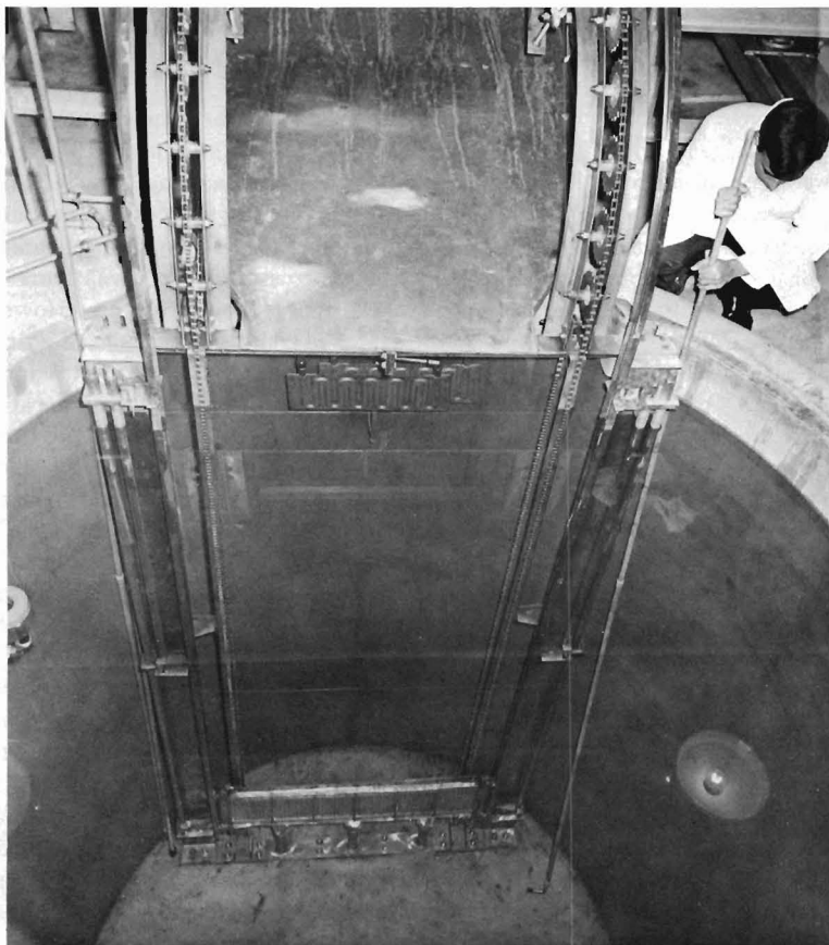
Pool of clear water at the bottom of which is stored the cobalt 60 (in the containers at the bottom of the track).
