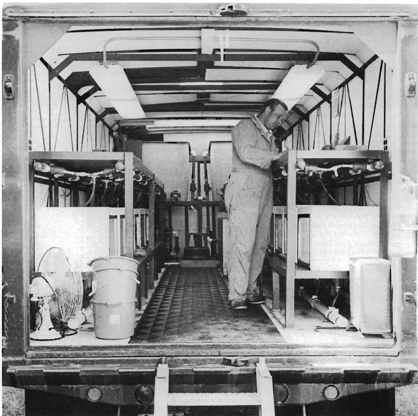
Figure 3.—Interior of mobile water temperature laboratory. Fishery biologist records observations as experiment progresses. Reservoirs for heated and chilled water are at forward end of van. Test tanks, supply lines, and temperature control valves are under counter tops. Drain lines are on floor under test tanks.
