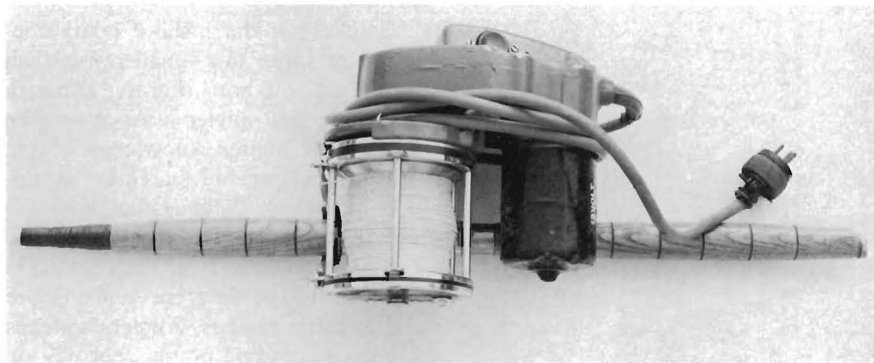
Electrically powered 9/0 reel as used in the headboat fishery. Photo courtesy of H. Gordy.
