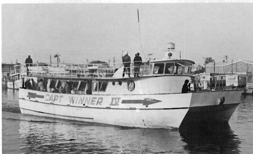
An aluminum hulled catamaran headboat at Carolina Beach, N.C. This type of vessel affords more comfort and angling space than conventional headboats, but the initial cost is great.
