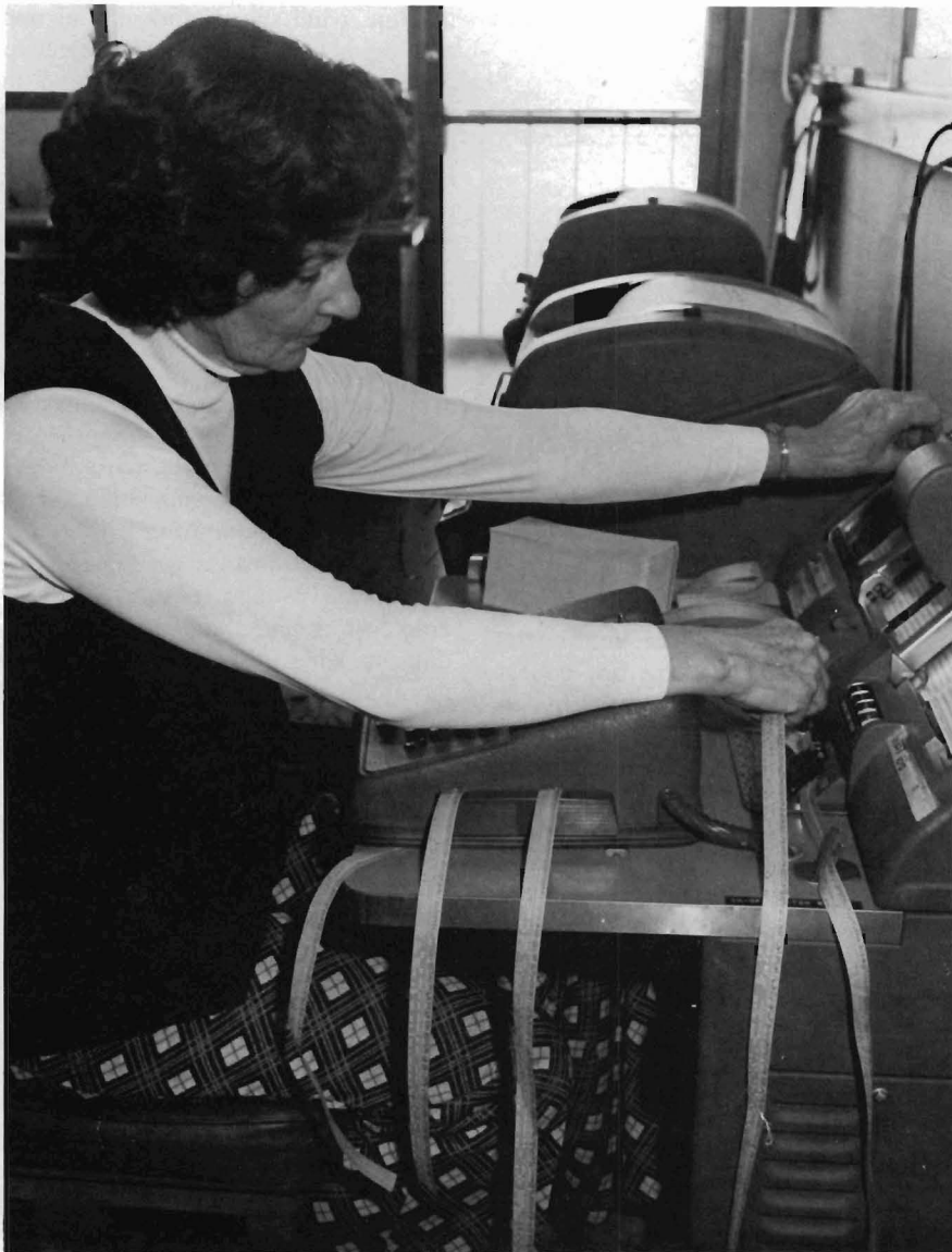
Figure 1.—Environmental data received over National Weather Service teletype circuits are recorded on paper tape, transferred to punched cards, and inspected for quality control. The cards are then used to update environmental data files on disk for computer processing.
