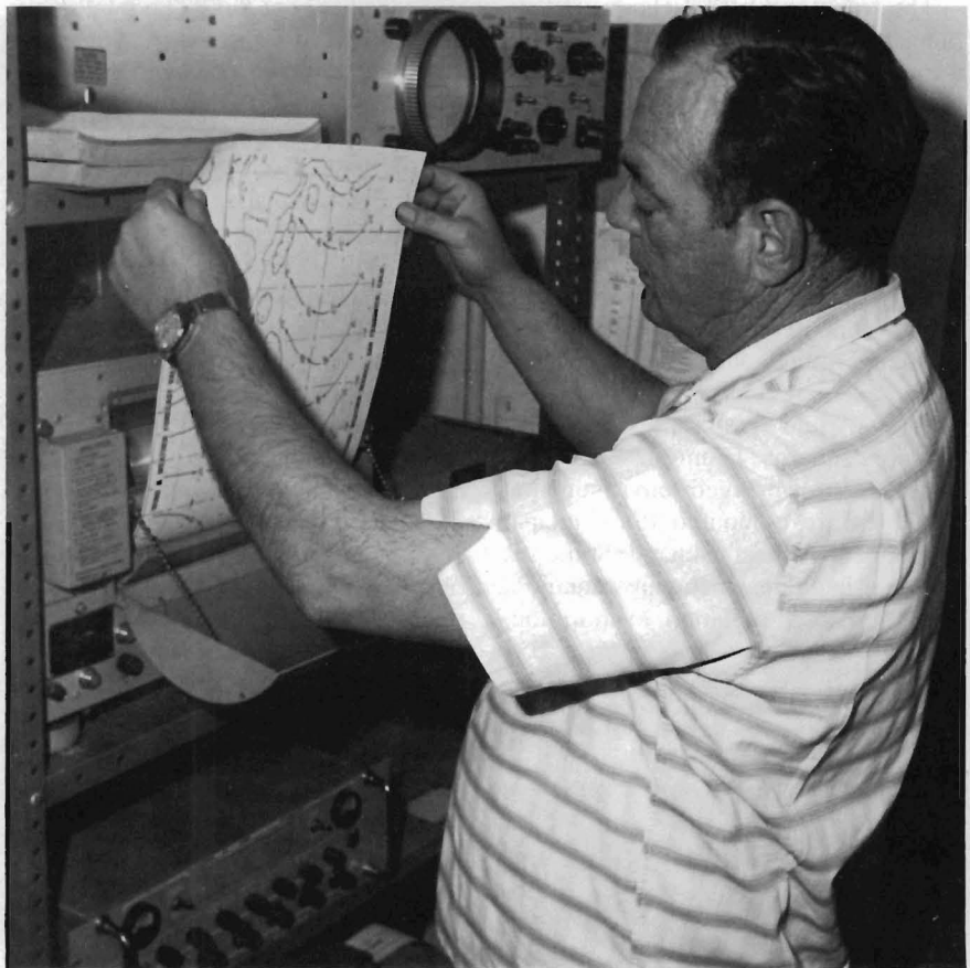
Figure 4.—Facsimile charts sent via land line from the San Francisco Weather Service Forecast Office are received simultaneously at the Southwest Fisheries Center and at radio station WWD, where they are recorded on magnetic tape. Visual inspection is made prior to transmission time for quality control.
