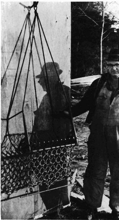
Figure 12.—A hand drag designed for harvesting oysters on soft leased areas. The thick toothed bar and runners prevent the drag from sinking into mud as it is towed.
