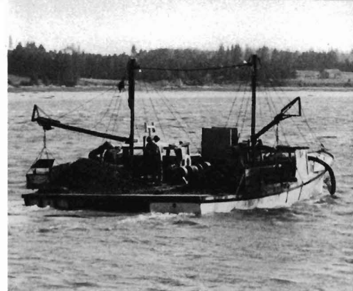
Figure 13.—Catamaran with part of an oyster load on its deck in East River. Note booms that lift drags.
