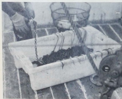
Figure 2.—A chain branch line with shark hooks attached.
