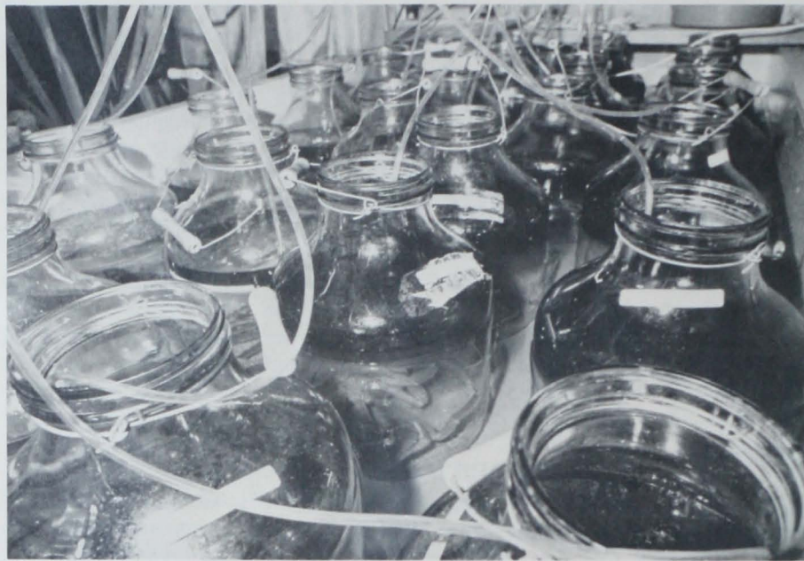
Figure 1.—Water bath and aerated containers used in static acute bioassays with crabs. Aeration tubes are glass-tipped to prevent contact of oil-water solution with tubing.
