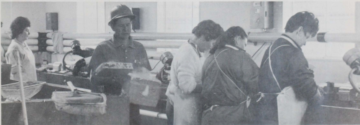
Figure 6. — Interior of marking shed near collection area where young fish are branded and wire tagged in assembly line. The fish are pumped into holding tank from raceways, anesthetized, and diverted to fish marking stations. After processing, the fish are transferred by gravity flow through pipe into tank truck.
