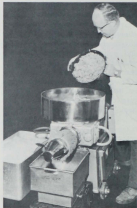
Figure 4.—Close-up view of Bibun strainer to show separation of minced flesh from skin or bone fragments.
