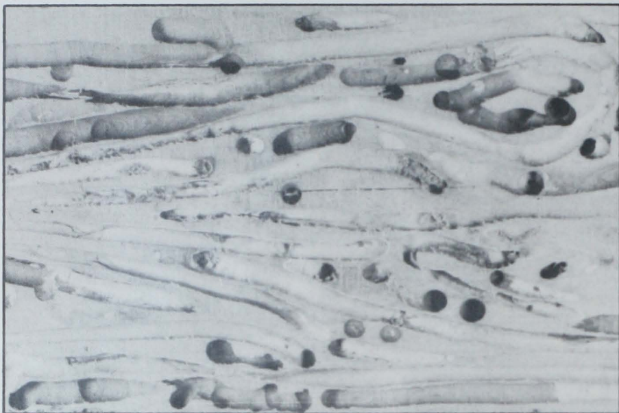
(Left.) A piece of fir showing the complete destruction of timber caused by the shipworm Bankia setacea . Burrows show calcareous lining secreted by the animal. Photograph by Dr. D. B. Quayle, Fisheries Research Board of Canada.
