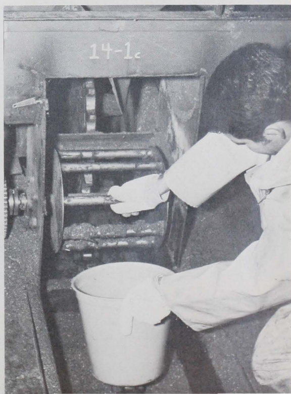
Figure 2.—A rotating grate magnet removes metal from scrap as the scrap drops from a conveyor.
