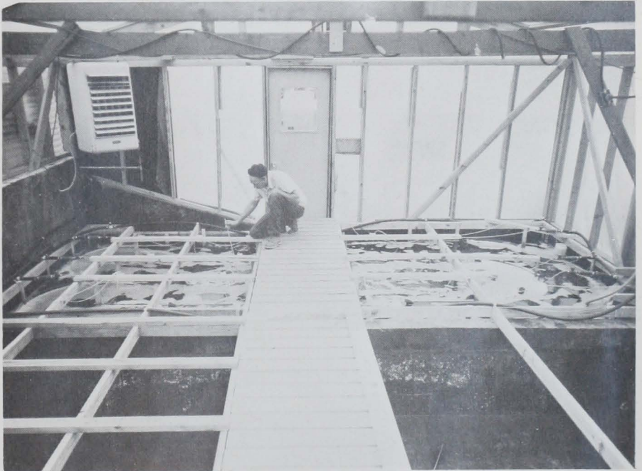
Experimental closed raceway system enclosed in a greenhouse to provide a controlled environment.
