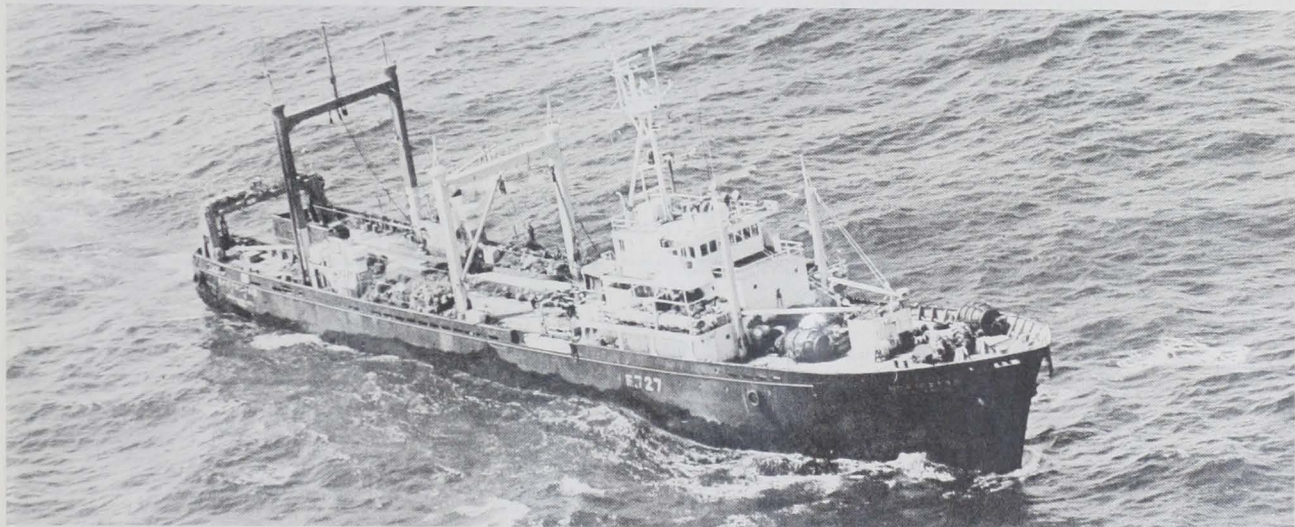
Fig. 9 - Medium stern trawlers (1,500 gross tons) are usually equipped with modern processing machinery, sharp freezers, and sufficient refrigerated holds to allow them to operate for some time without support.
