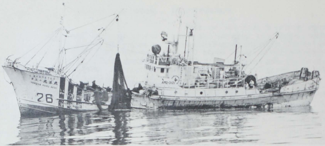
Fig. 5 - Brailing fish from the net on a Danish seiner in the eastern Bering Sea. Danish seiners, like most side trawlers, fish in fleets with a factory ship which processes their catches.
