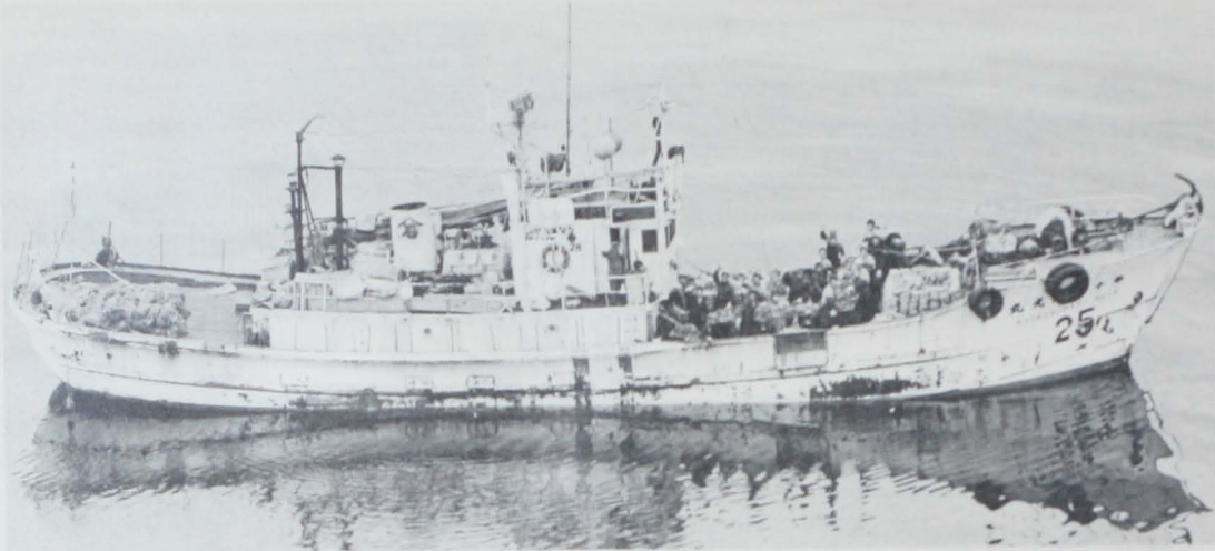
Fig. 17 - Tanglenet fishing vessel operating in the Japanese crab fishery of the eastern Bering Sea. As the tanglenet is brought aboard, the crab are removed and placed in large cargo nets for transfer to the factory ship.
