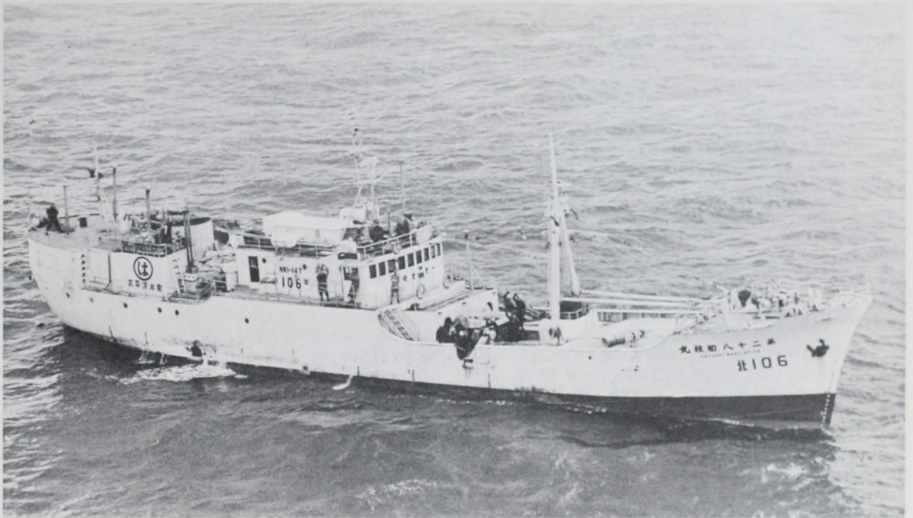
Fig. 12 - Japanese longliner fishing in the Gulf of Alaska. This ship is typical of the older style longliner with the open work area on deck.
