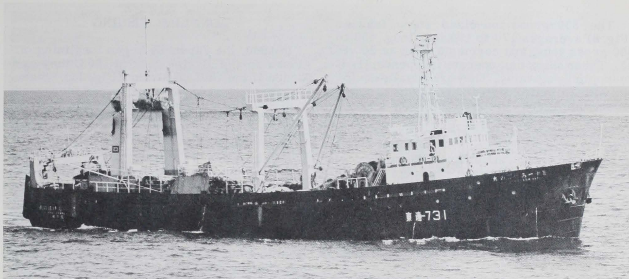
Fig. 8 - A stern trawler of this size (500 gross tons) is designed for independent operations. Processing usually includes only heading and freezing. This type of stern trawler is used in many areas off Alaska.
