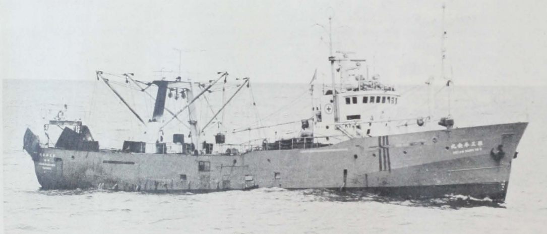
Fig. 7 - Small stern trawlers of this design usually work in fleet operations with a factory ship. Although some of these small stern trawlers have limited processing equipment which would enable an independent operation, they must then work in an area where resupply is readily available.
