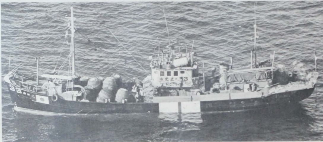
Fig. 18 - Crab pot fishing vessel (dokkosen) used in fleet operations by the Japanese in their crab fishery. Conical shaped crab pots used extensively by the Japanese for Tanner crab are visible on board.
