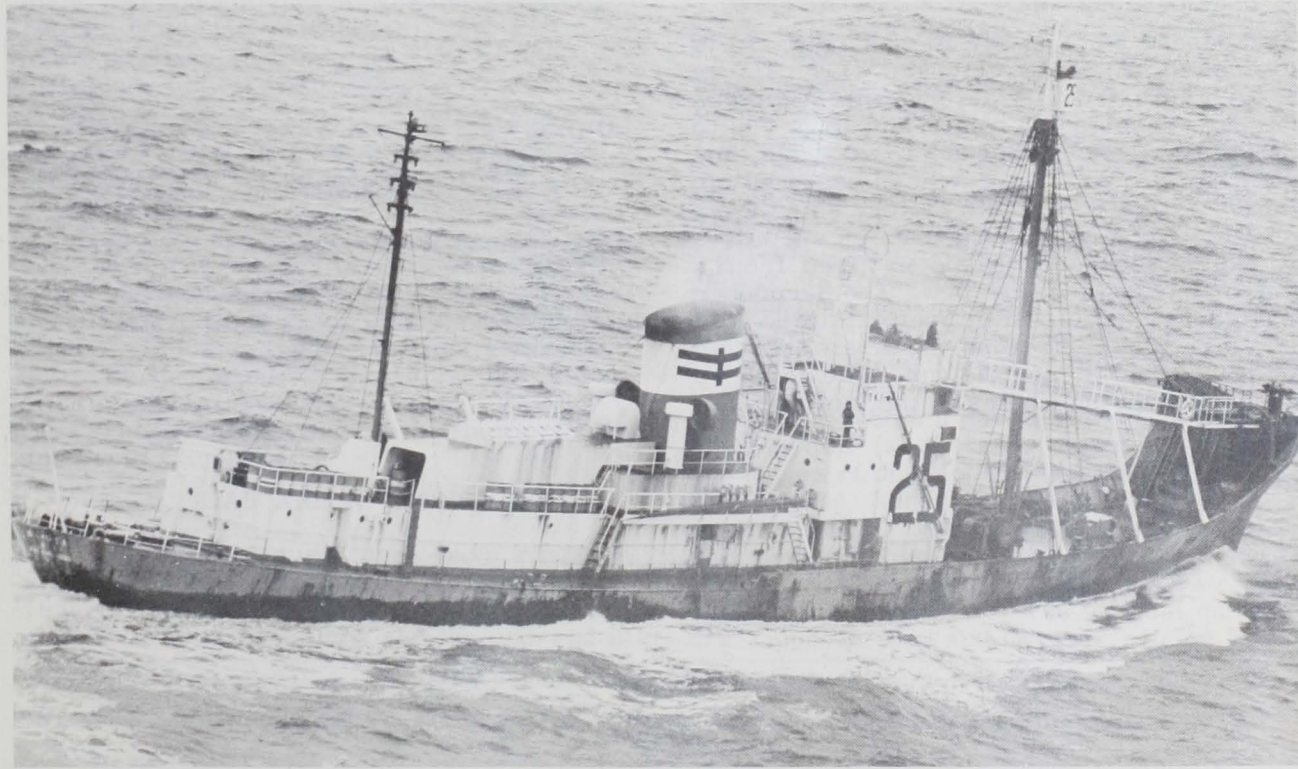
Fig. 21 - Whale catcher of the type used off Alaska. Note the catwalk used by the captain or harpooner to get from the bridge to the bow and the harpoon gun mounted on the bow.
