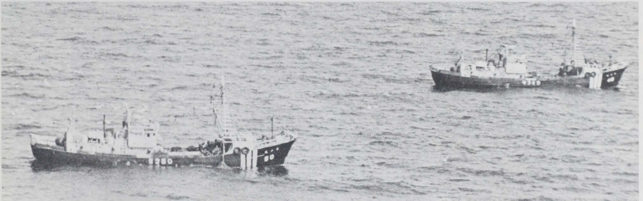
Fig. 3 - Pair trawlers fishing in the eastern Bering Sea. The two vessels operate together towing one trawl. Pair trawlers, like side trawlers and Danish seiners, operate in fleets with a factory ship.
