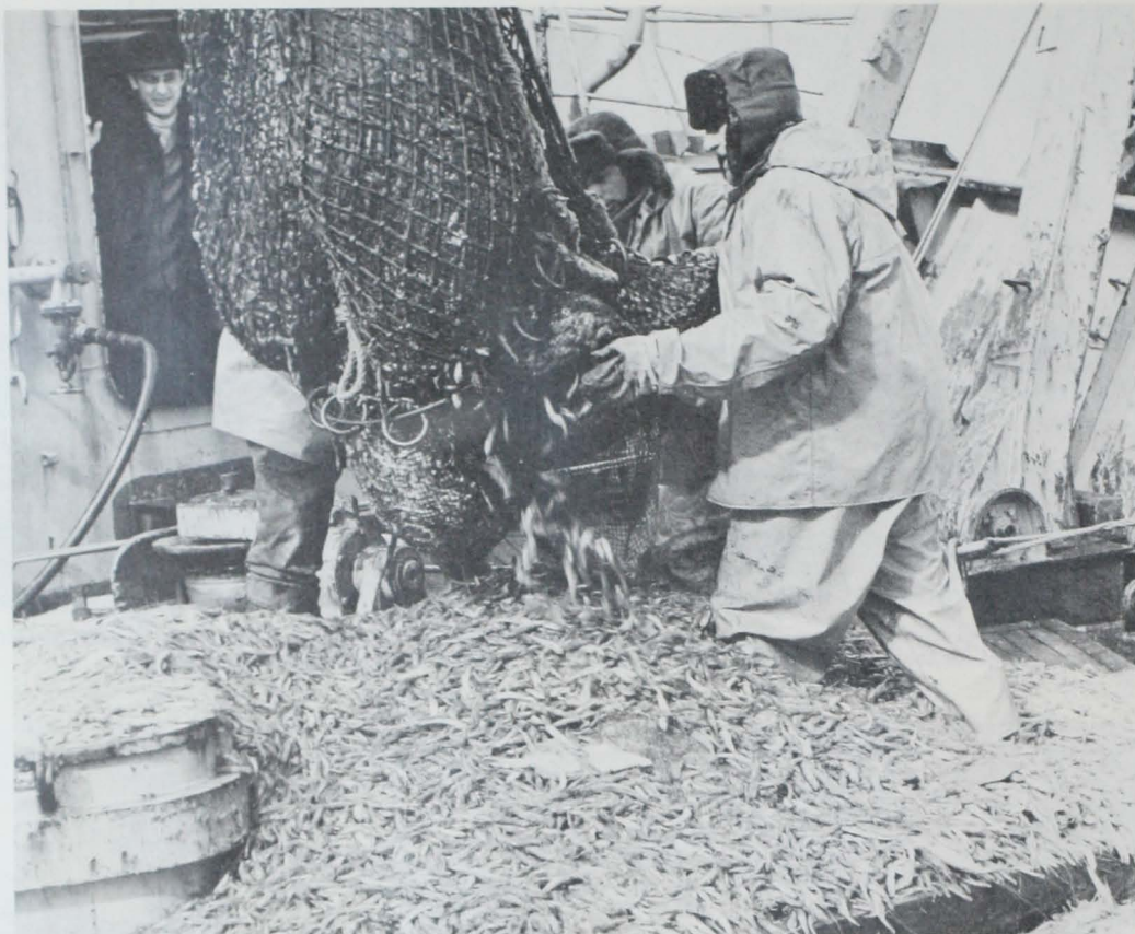
Fig. 4 - A 2,000-lb catch of pink shrimp being dumped on deck. The \frac{3}{4} -inch mesh liner inside the cod end can be seen extending past the puckering rings.
