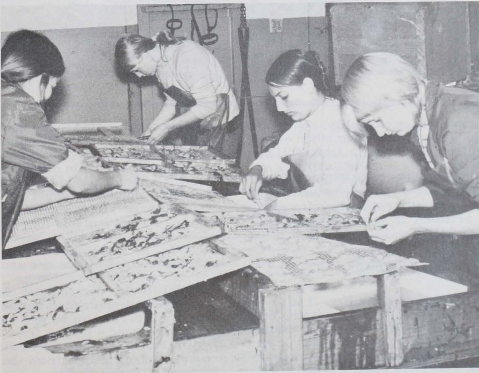
Fig. 5 - Sea urchin roe are drained on a wire screen.
