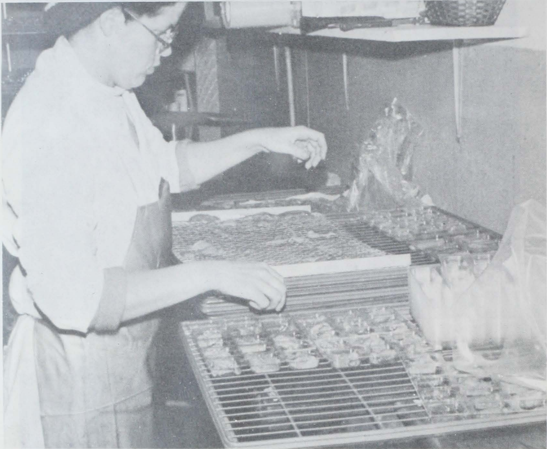
Fig. 6 - Plastic trays with compartments for individual roe are used for packing.
