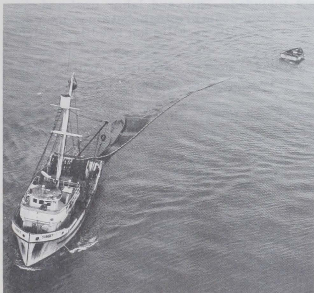
Fig. 5 - The start of a set. Skiff has been dropped and net drum is free wheeling. (R. Green)
