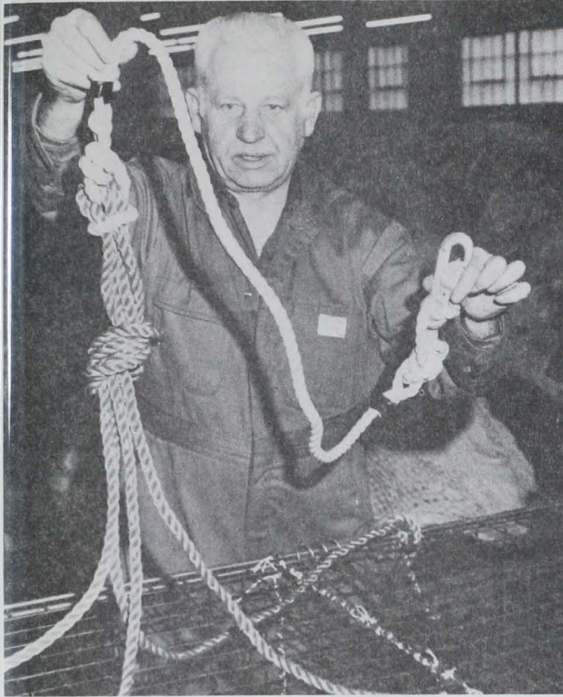
Fig. 4 - A spring-loaded snap hook at the end of the bridle permits the trap to be quickly connected or released from the groundline. Small rope loops (beckets) are placed at intervals (commonly 50 fathoms) in the groundline to space traps evenly.
