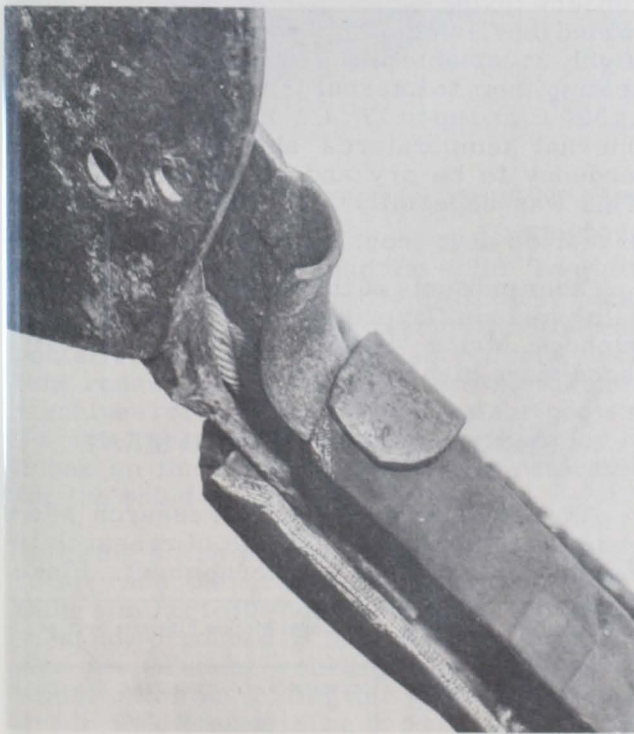
Fig. 4 - Discharge hose and lower end of guiding channel showing the slot for threading and removal of line. (Photos: William L. High)
