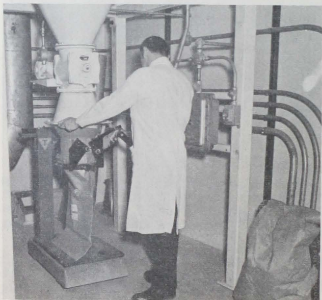
Fig. 9 - Pulverized FPC is milled and bagged in a separate room.
