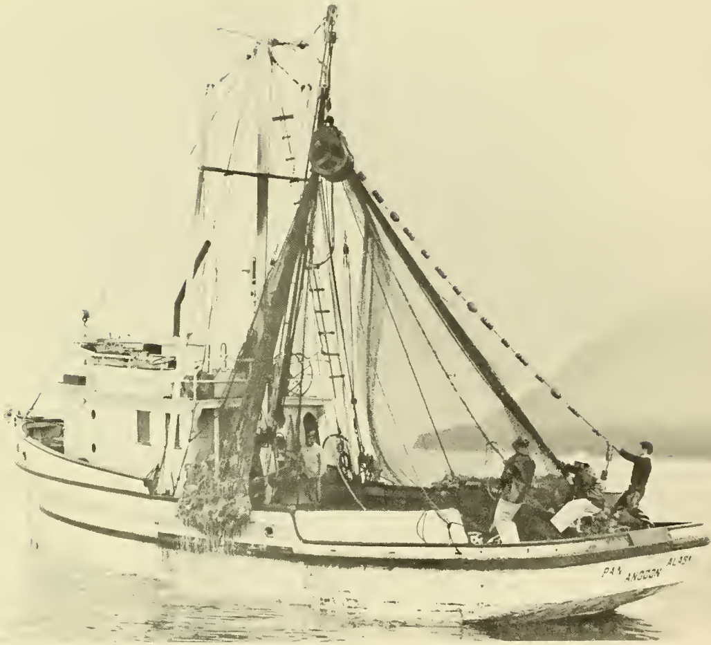
Figure 5.—Hauling in the net on a pink salmon purse seiner. When set for fishing, the net encloses an area of about 2 acres.
