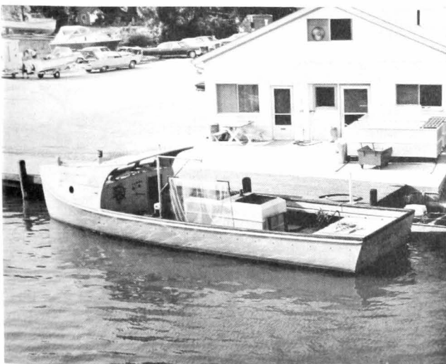
Figure 2.--A typical vessel used in the bait minnow industry. Note the vessel has live tanks for storing the catch and a davit for handling the lift net.
