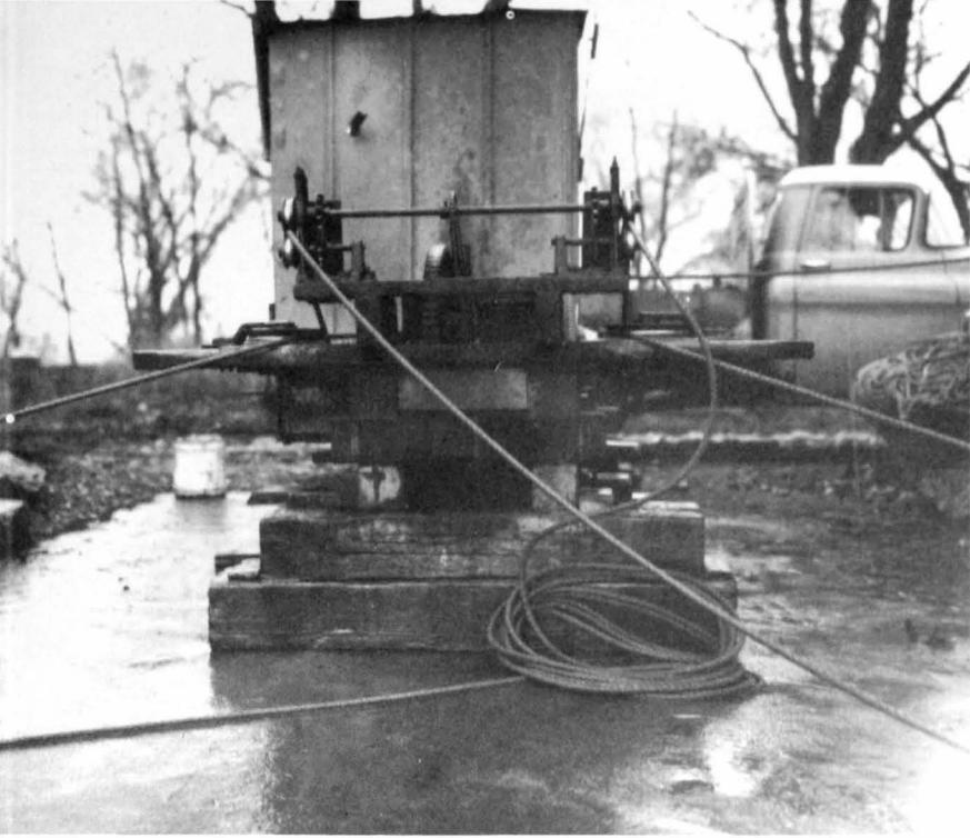
Figure 8.--Seine winch installed on shore at permanent fishing site. Note the operation of the coiling mechanism.
