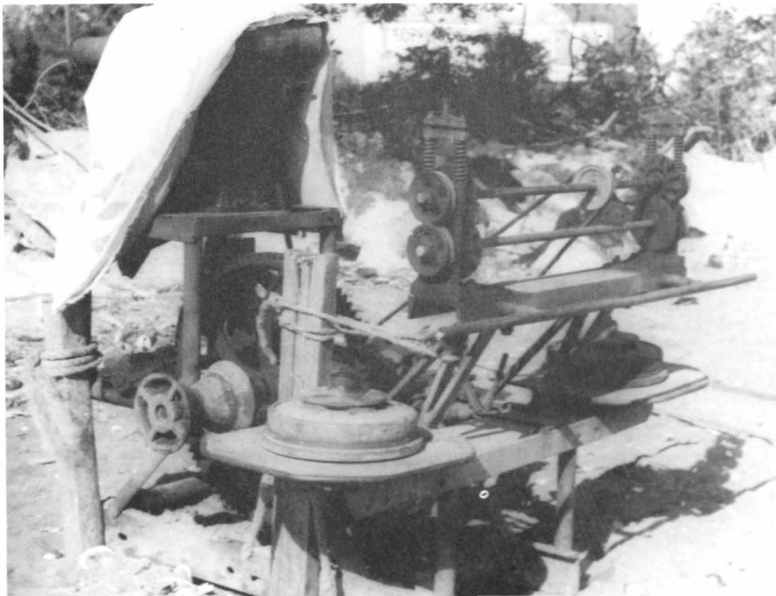
Figure 9.--Portable seine winch anchored along each ready for fishing.
