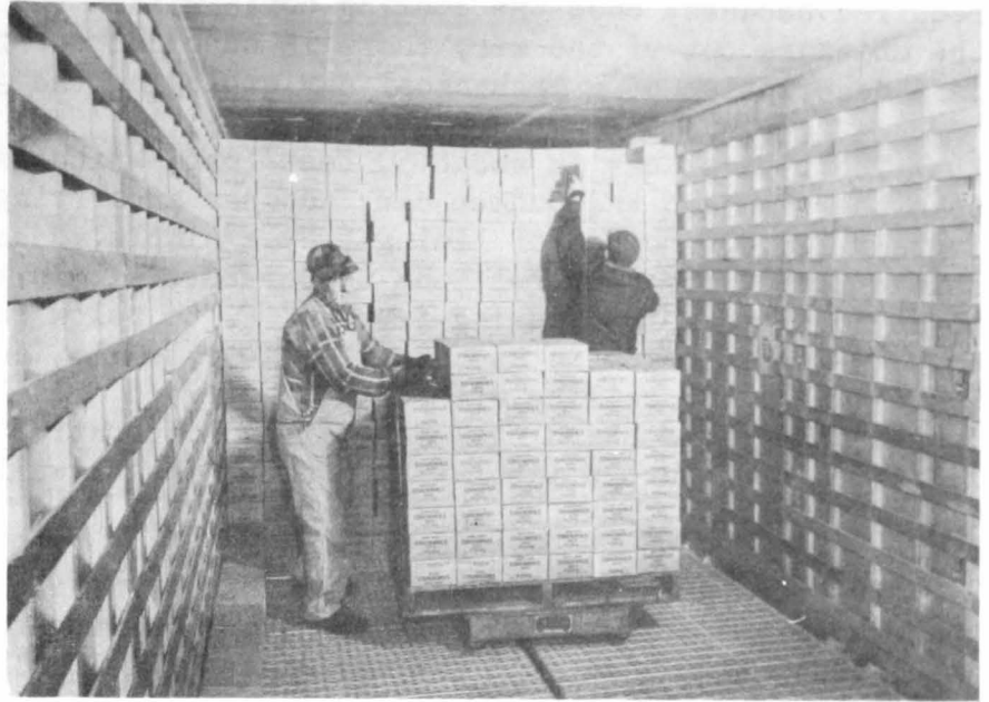
Figure 10.—Inside view of a mechanical refrigerated car. In this car, cold air circulated in a duct between the ceiling and the insulation, by fans, enters the product storage space through holes located in the ceiling. (Photo courtesy of Santa Fe Railroad)
