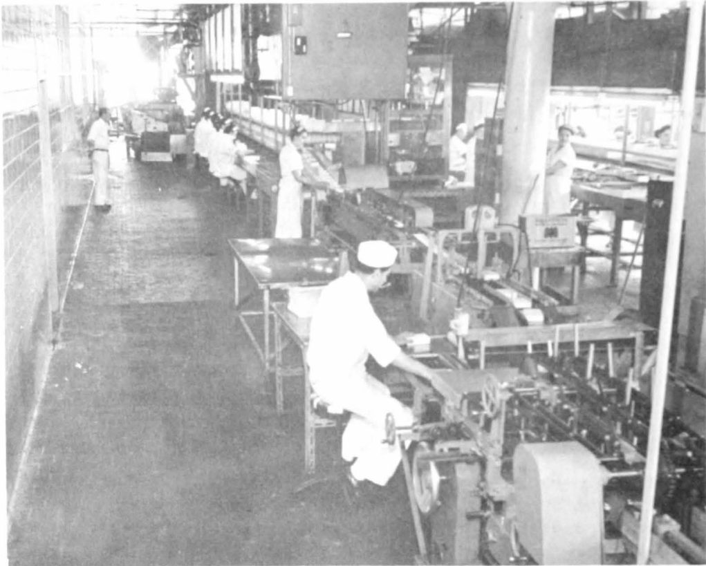
Figure 19.--View of packaging line and automatic overwrapping of packages. (Photo courtesy of The Great Atlantic and Pacific Tea Company)
