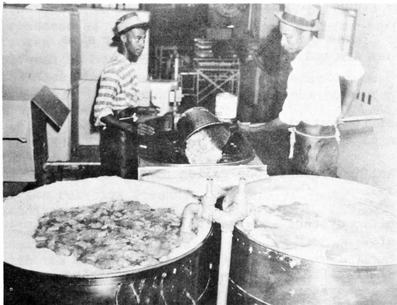
Figure 3.--After the oyster meats are removed from the shell, they are washed by being "blown" in large tanks of water. (Photo courtesy of Southern Fisherman)
