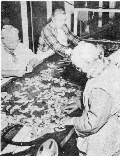
Figure 7.--Upon coming into the plant, the shrimp are inspected and defective ones removed. (Photo courtesy of Southern Fisherman)
