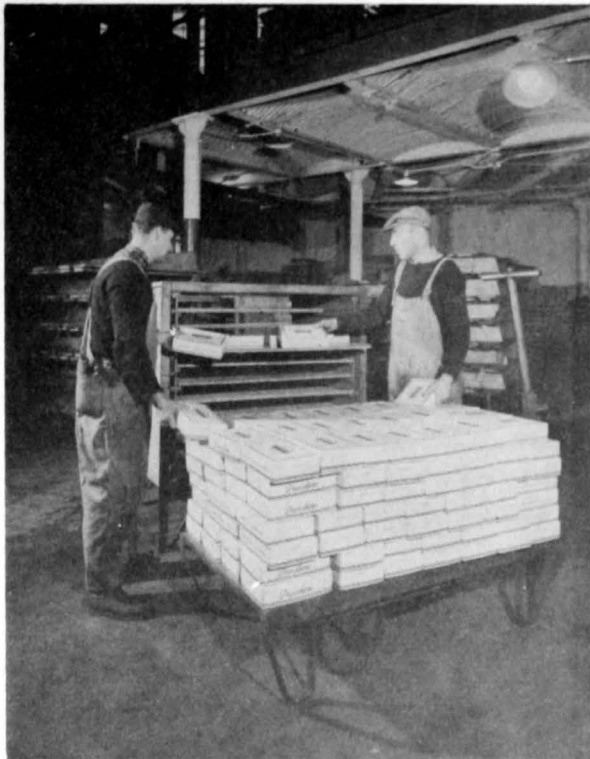
Figure 8.—Loading 5-pound packages of fish on a blast freezer rack. (Photo courtesy of Quincy Market Cold Storage and Warehouse Company)
