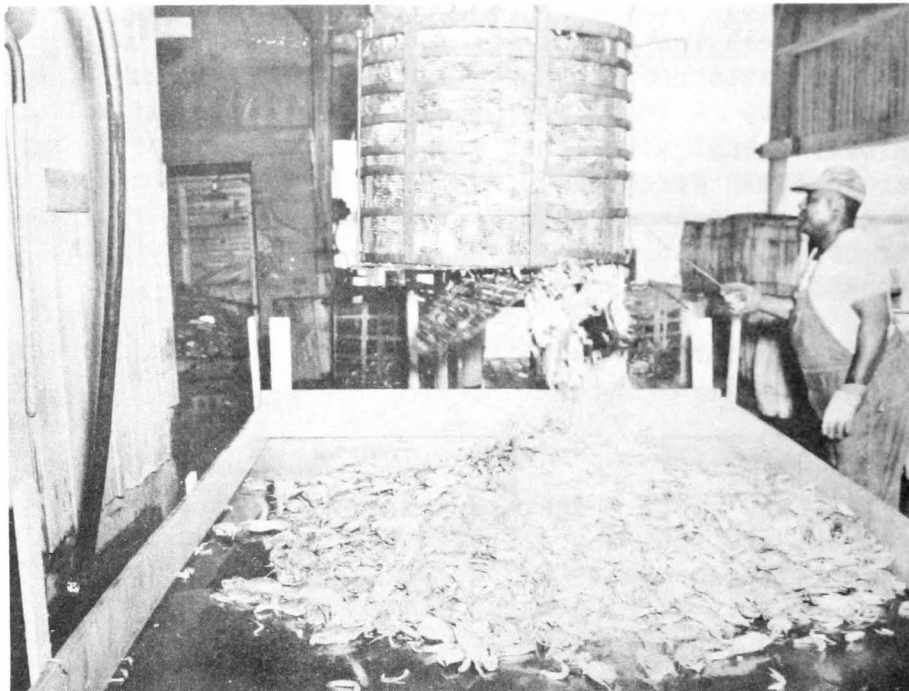
Figure 14.--Cooked crabs are dumped onto a platform to cool prior to having the meat removed. (Photo courtesy of Southern Fisherman)
