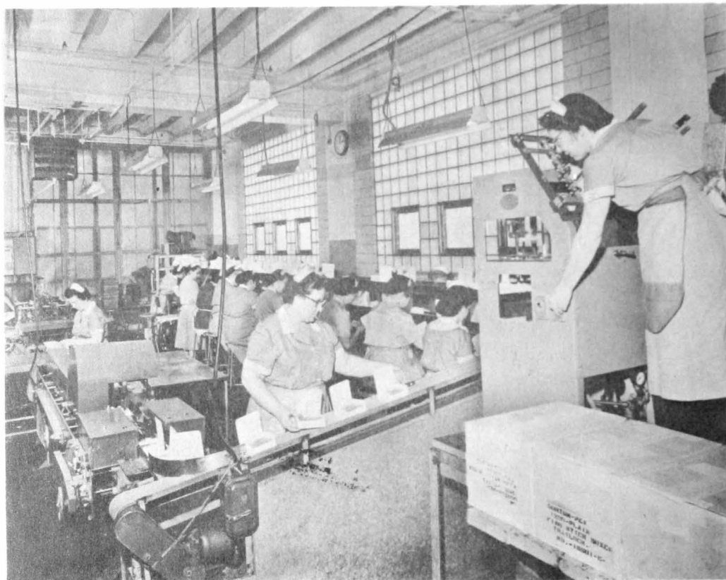
Figure 6.--Formed cartons are filled on the packing table (background), and pass quality control inspection (foreground) prior to being automatically closed and wrapped (left). (Photo courtesy of Package Machinery Company.)
