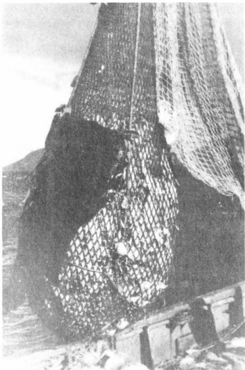
HOISTING THE BAG ABOARD. COWHIDE CHAFING GEAR WAS USED TO PROTECT THE BAG FROM ABRASION.
