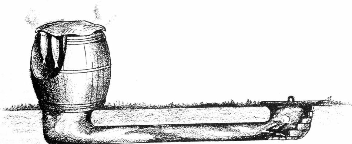
Barrel Smokehouse with Fire Pit at a distance for Hot or Cold Smoking
