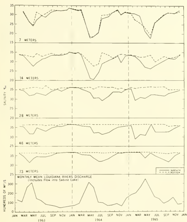
Figure 3.—Salinity trends in surface and bottom waters over the continental shelf off Louisiana, 1963-65.
