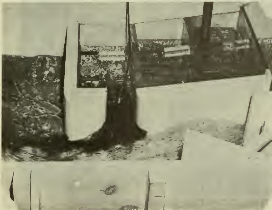
Figure 15.-- Entrance to Fishway (Model) Tailwater Elevation 11 ft. (above mean sea level) This water level is probably close to the minimum tailwater level for entrance of shad into the fishway. Note that the first weir is flooded.
