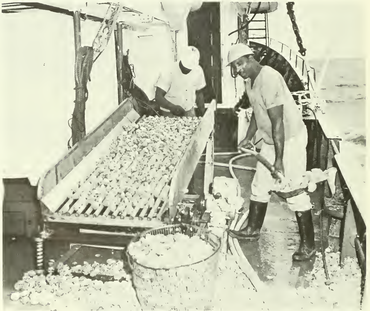
Figure 16.—Culling machine for separating live scallops from shells and debris being tested aboard the exploratory fishing vessel.
