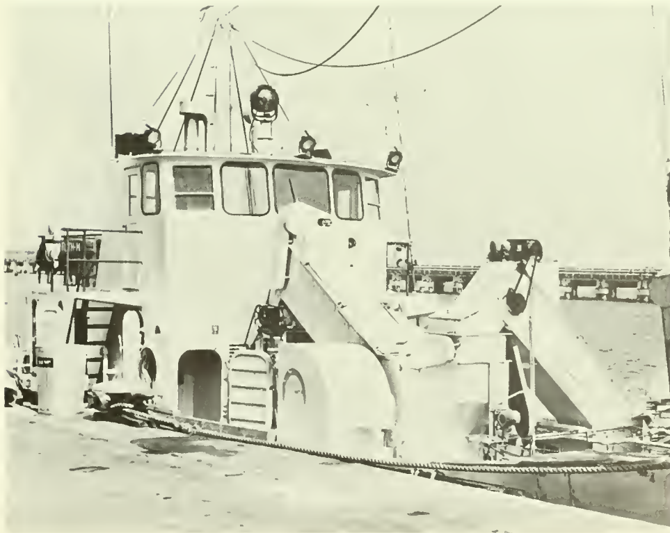
Figure 14.—Commercial size shock-heat-shocker shucker installed aboard 136-foot fishing vessel.
