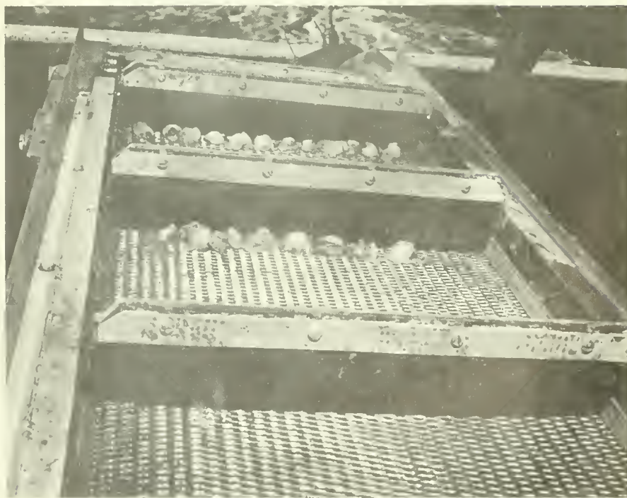
Figure 10.—Prototype experimental eviscerator being tested aboard the exploratory fishing vessel.
