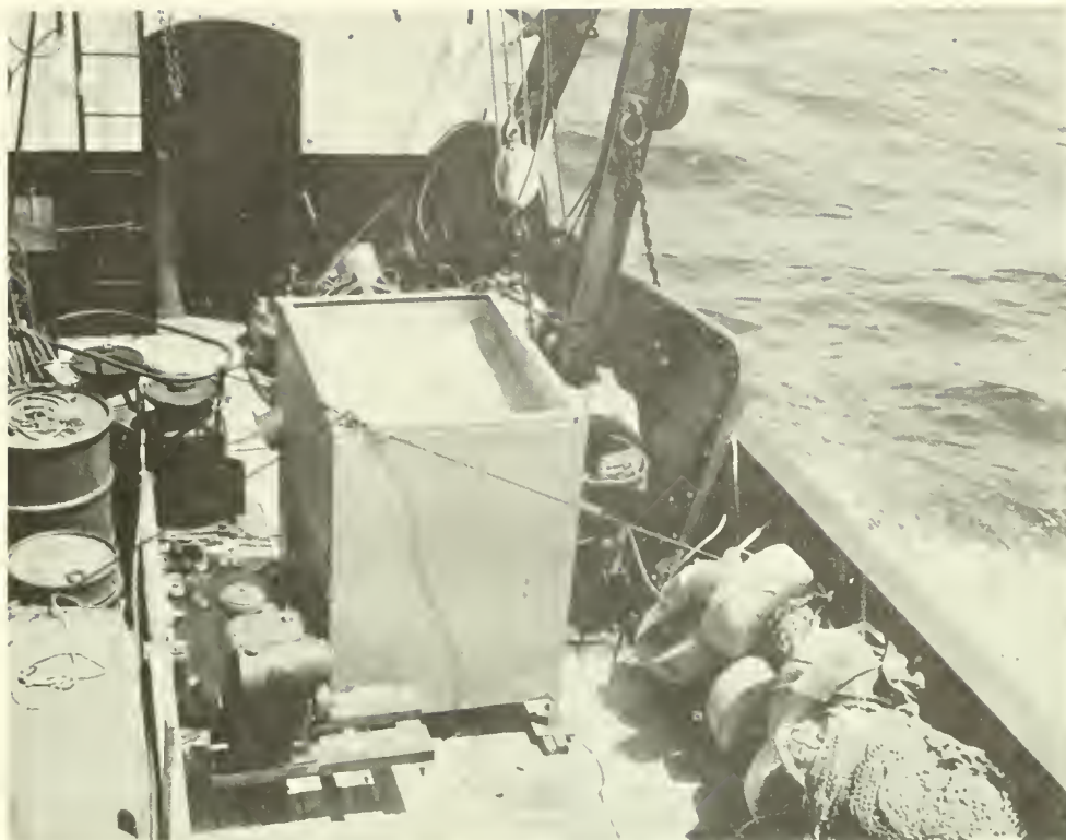
Figure 9.—Experimental combination shucker and eviscerator aboard the exploratory fishing vessel.
