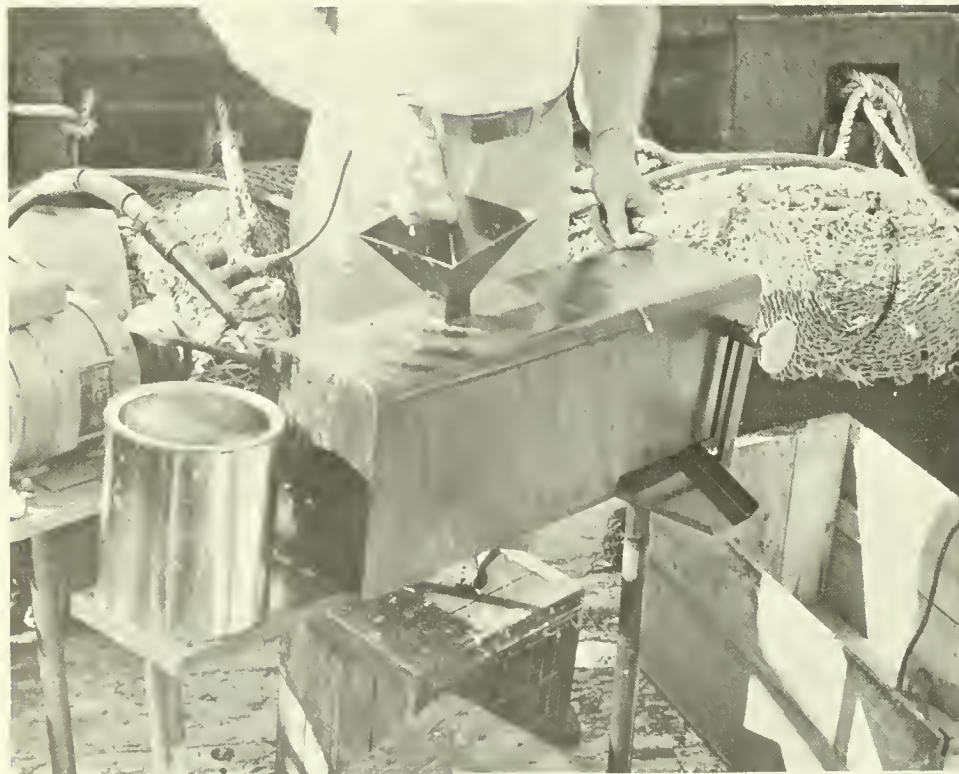
Figure 8.—Prototype experimental eviscerator being tested aboard the exploratory fishing vessel.
