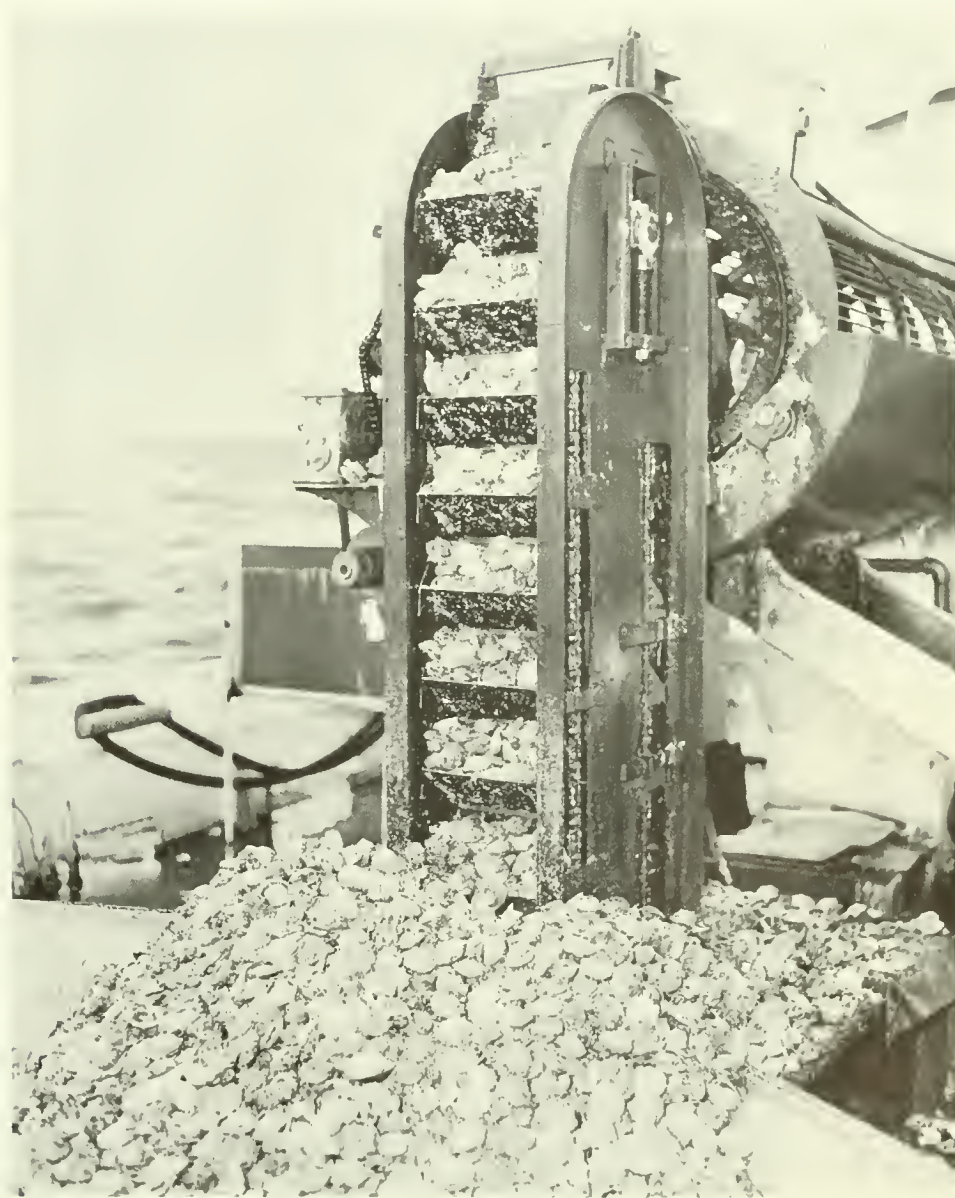
Figure 17.—Bucket conveyor and rotary "squirrel cage" type culling machine, for sorting live scallops from the catch, installed aboard 86-foot factory-type scallop vessel.
