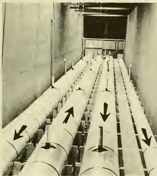
Figure 3.--The 82.3-m.-long, 0.6-m.-diameter pipe system (three sections on left) and the 27.4-m. section of the 0.3-m.-diameter pipe (on the right), 1964. Arrows indicated direction of flow. Fish entered pipes downstream of area in foreground and exited upstream of wall in background. Small upright pipe extensions contained lamps.
