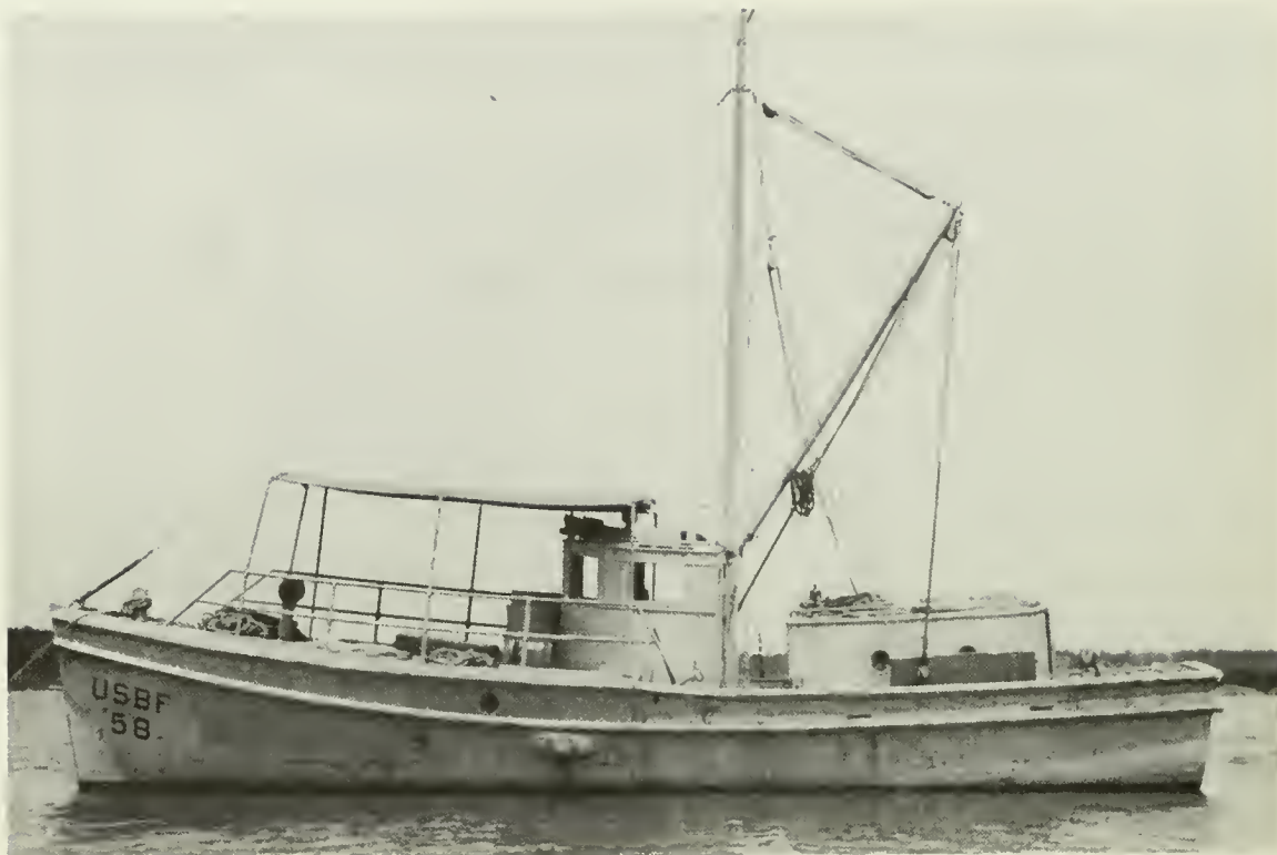
Figure 1.-- Launch 58 , a 40-foot (12.2-m.) shrimp trawler used in the studies of white shrimp along the south Atlantic coast in 1931-35.
