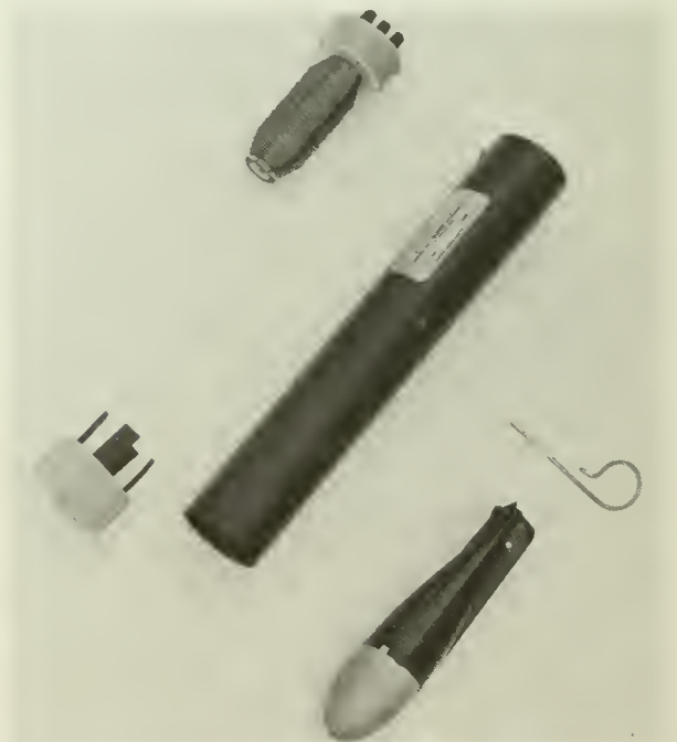
Figure 3.--Disassembled canister. The shipboard end of the fine wire pays off the spool (top center) in the canister (center) while the end connected to the thermistor pays from another spool inside the probe (lower right) through the finned end. Water enters the tube at the tip of the weighted nose of the probe, flows past the thermistor and out through the same orifice as the wire. The cap (left center), removed before loading into the launching tube, provides rubber cushioning to protect the thermistor during shipment and handling. The pin (right center), inserted through the holes in the canister and the hole in one fin of the probe, locks the probe in the canister. When the pin is pulled, the probe is released and slides out of the launch tube by gravity.
