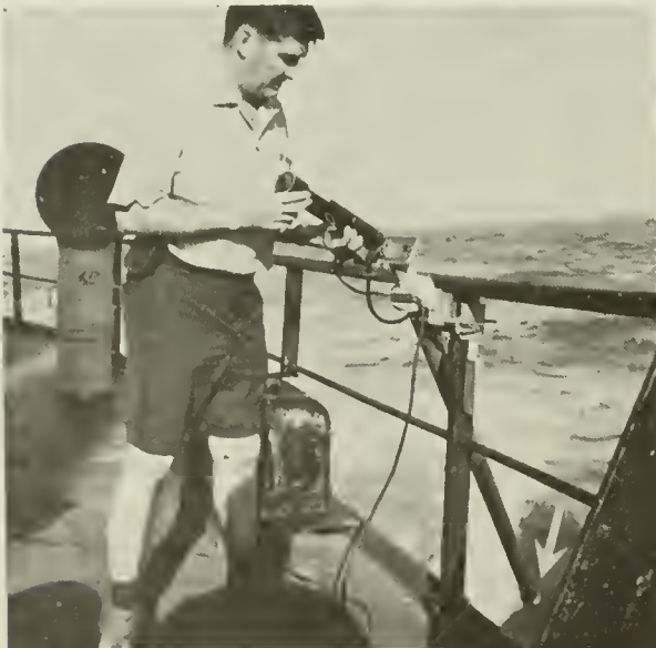
Figure 1.--Placing an expendable thermograph canister in the loading breech of the launcher. The arrow is pointed at the lower end of the discharge tube.
