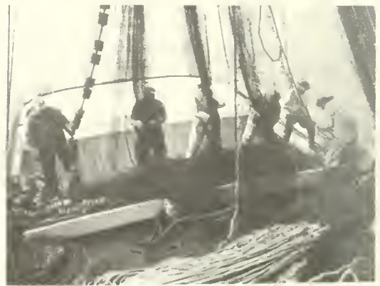
⑩ Webbing being piled on stern by crewmen as it descends from power block
