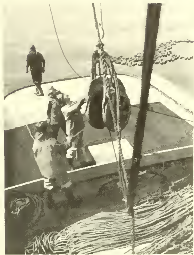
⑦ End of net being threaded through power block
