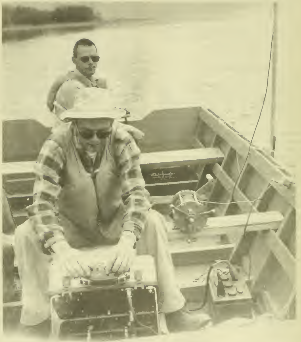
Figure 32.--Sounding Brooks Lake with portable echo sounder. Transducer rod is on right, over side of boat. Point of land in background is reference point (transect 41).
