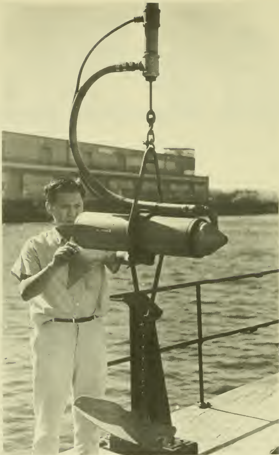
Figure 2.--The collector mounted in the diamond-shaped bridle with the hose-cable terminal assembly above and the depressor below.
