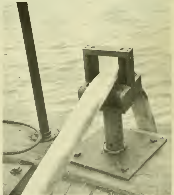
Figure 7.--The guide wheel, composed of 2 horizontal rollers and 2 vertical rollers. It is mounted on a short vertical post and rotates freely in the horizontal plane.
