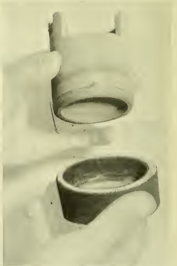
Figure 10.--The collecting bucket with the friction cap detached. The edge of the bucket is recessed to accommodate the tension screw of the steel clamp on the neck of the funnel. The rubber "O" ring on the neck of the funnel seals the bucket below the edge of the large recess.
