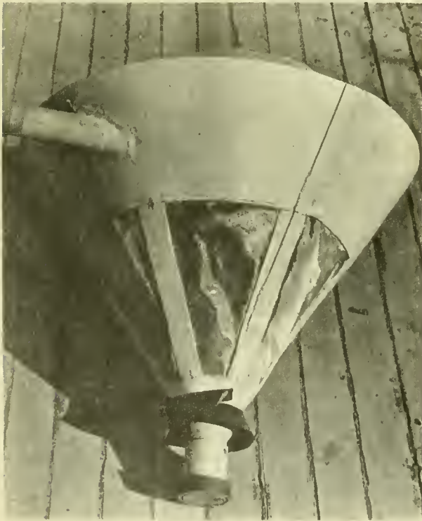
Figure 9.--The filtering funnel with the bayonet mounted collecting bucket and the friction fitted cap in place.
