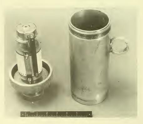
Figure 2.-- Assembled bathykymograph with cover removed.
