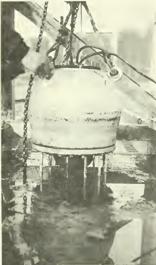
Figure 6.-- Audio speaker used to produce low frequency sound, (Here shown out of the water.)
