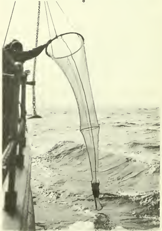
Figure 10.--(Above) Net for collecting micronekton at 5 knots. (Below) Net for collecting micronekton at 10 knots.
