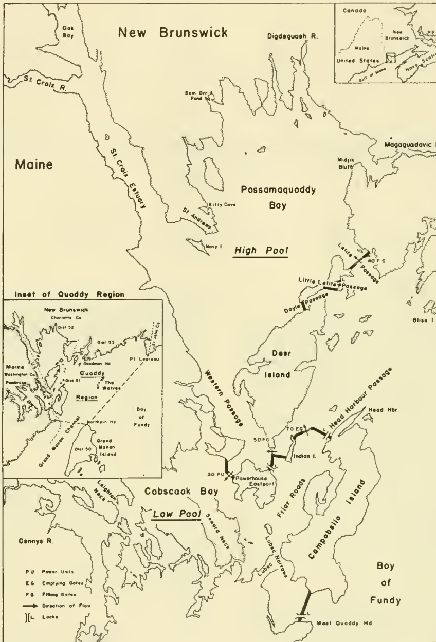
Figure 1.--Map showing location of high pool, low pool, filling gates, emptying gates, and powerhouse. The Quoddy Region is shown in inset.
